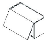
Hanging Swing Door Cabinet Width: 500 / 600 / 700 800 / 900 / 1000 Depth: 450 Height: 500
